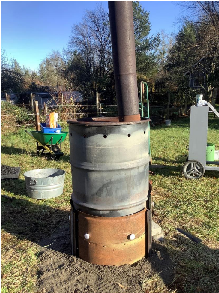
Two-Barrel Nested Biochar Retort—Prior to Burning
